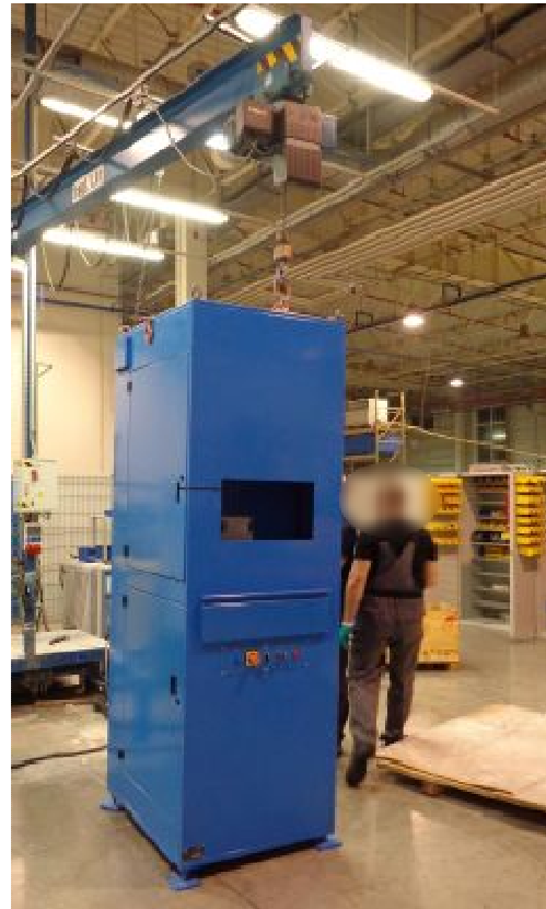
Figure 14: Cabinet lifting process using the rings
